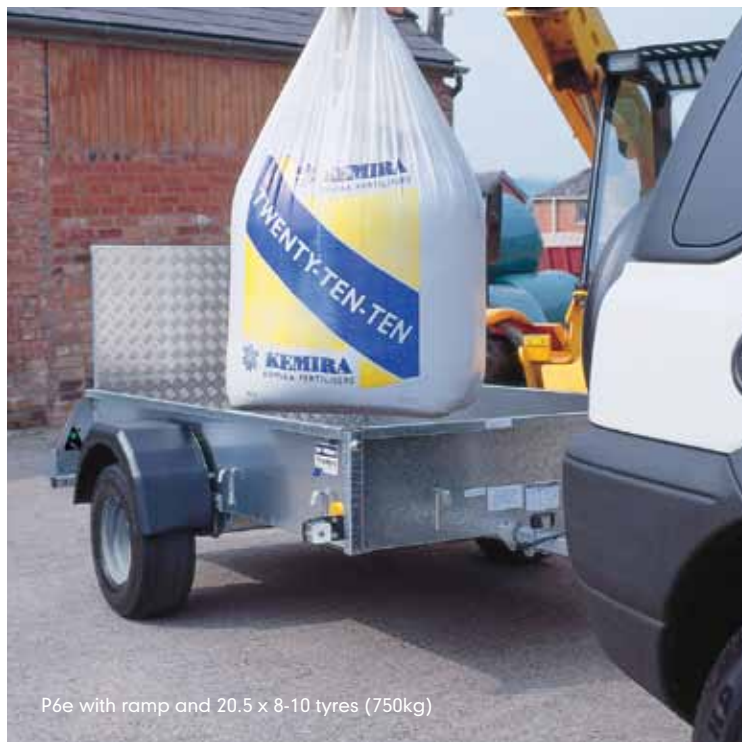
P6e with optional stock ramp door, weldmesh panelled sides and 20.5 x 8-10 tyres (750kg)
